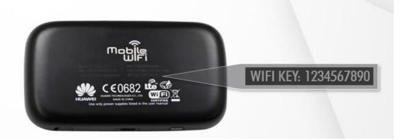
Or you can press the WPS button 4 times, which will display the Wi-Fi KEY
