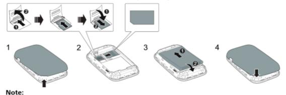
• Make sure if it's for a Prepaid client that you activate the SIM first by making a call and deactivate the SIM PIN before you insert the SIM in the Mi-Fi.
